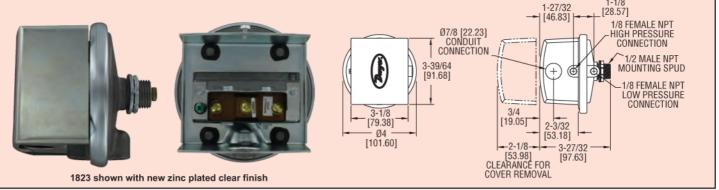
Essential for industrial environments, the Series 1800 combines small size and low price with 2% repeatability for enough accuracy for all but the most demanding applications. Set point adjustment inside the mounting stud permits mounting switch on one side of a wall or panel with adjustment easily accessible on the opposite side. UL and CSA listed, FM approved.
