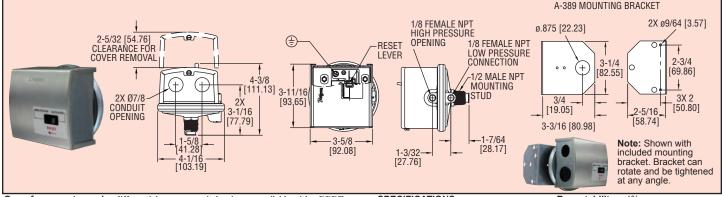
**One of our most popular** differential pressure switches is now available with a DPDT switch and manual reset. The 1831 combines small size with 4% set point repeatability. Absolutely no power is required to operate the DPDT switch. Set point adjustment on the switch is easily accessible for modifying the set point.
