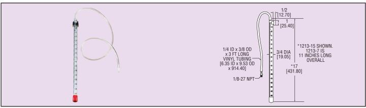
**Provide visual indication of pressure** with the Series 1213 Gas Pressure Manometer. Designed for use with natural gas, the manometer can also be used to monitor any compatible gases up to 15 inches of water column. Tap water is used as the sensing media and a magnetic clip provides temporary or permanent mounting. Economically priced and made of durable plastic for years of trouble-free service. Includes 3´ of vinyl tubing and 1/8″ nylon male NPT to barb fitting.
