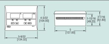
Simultaneously measure and control temperature and humidity with the Series THC Temperature/Humidity Switch. The unit offers a 3-digit red display for temperature indication and a 3-digit green display indicating humidity. The Series THC is equipped with four independent relays, two for temperature control and two relays for humidity control.
