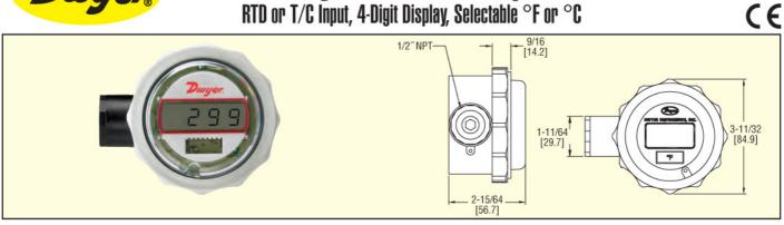
The Series BPI Battery Powered Indicator  $accepts\ RTD$  or Thermocoupleinput and provides local or remote display of temperature measurements. Quickly navigate the menu system to customize for each application. Three push buttons allow the user to select input type, engineering units (°F or °C), offset temperature, decimal point position, and password protection. The indicator is housed in a polycarbonate NEMA 4X (IP66) enclosure for additional protection from the environment.
