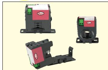
The Series SCS Low Cost Current Switches are ideal for monitoring whether fans. pumps, or motors are operating. The current flowing through the core of the device powers the circuit without an external power supply. All models have a built in solid state output and are easy to install. Optional LED's and 10 Amp relay modules are available. The Series SCS is available in both split and solid core configurations.
