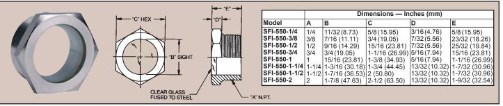
Fused glass style sight windows feature glass to metal bond for utmost reliability. Plated steel bodies have convenient hex wrench surfaces. Connections are standard NPT in sizes from 1/4 " to 2". Windows are clear, ripple free, and flush with the front face, having no recess on which dirt might collect.
