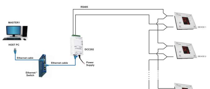
\* Use Ethernet Switch with PoE to eliminate power supply connection to DCC202
