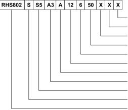
**Optional accessories** No. of calibration points Termination (ref. table 2) Insertion Length Sheath Dia (ref. table 3) 1/2" Tri-clover (ref. table 1) Class A accuracy Pt-100, 3-wire Terminal head No. of circuit
